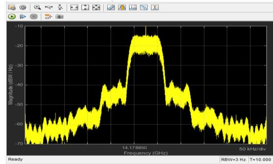
Figure 7: Transmitted Signal Power Spectral Density (PSD)
