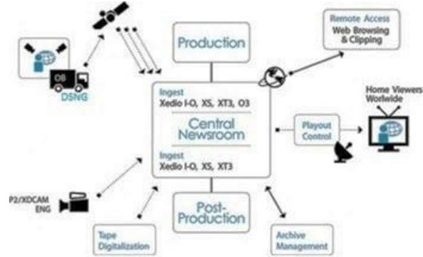
Figure 1: Block Diagram of Operational Department in a Digital Television Channel
