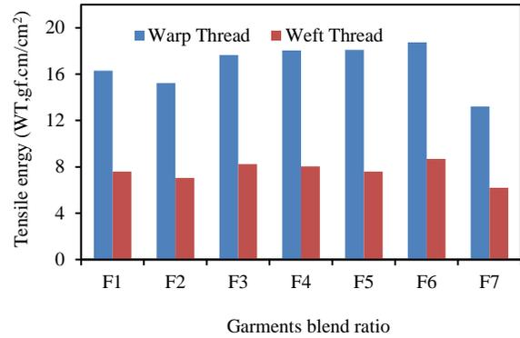
Figure 2. Tensile energy of Bamboo: Cotton blended garments
